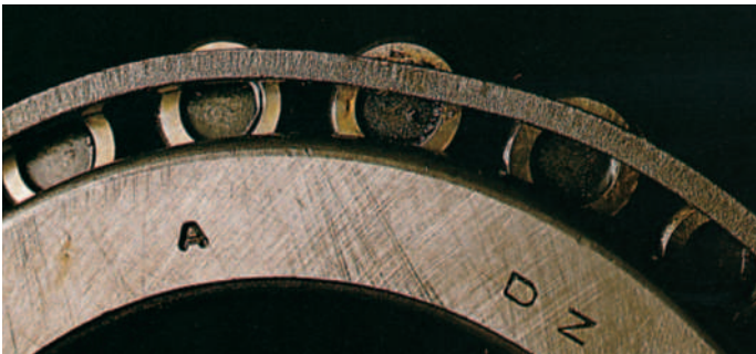
Deformation of the cage, the result of improper installation or mishandling prior to installation.
