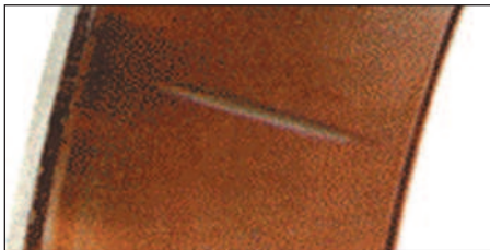
Dent across the race indicates a sharp high impact.
