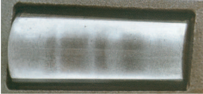
Uneven wear on the roller, the result of improper installation.
