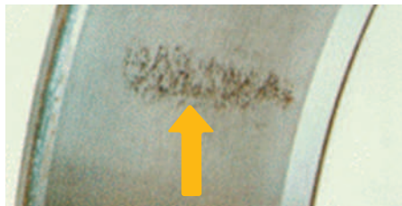
Etching of metal generally indicates water contamination, allowing oxidation to attack the surface.
