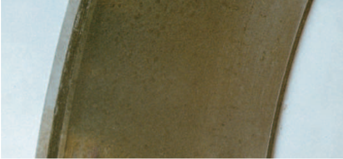
Peeling, the tearing away of metal from the race, the result of the breakdown of lubrication.
