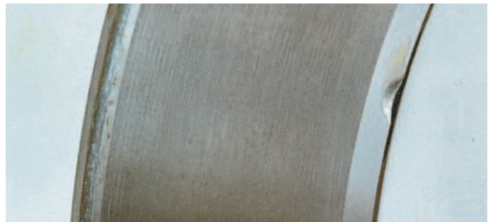
Damage to the cup front face, the result of installation damage through use of a hardened driver.
