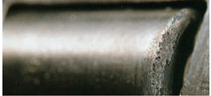
Large end of the roller shows spalling, the result of insufficient lubrication and/or excessive preload.
