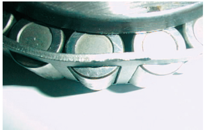
Examine the inner ring raceway by holding the bearing against a light and turning the cage slowly. Look for pitting, flaking, discoloration and corrosion.
