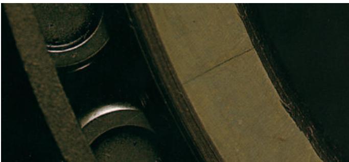
Cracked cone, the result of misapplication or cocking the cone at installation.
