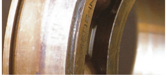
Discoloration indicates high levels of heat, the result of improper lubrication or improper bearing adjustment.
