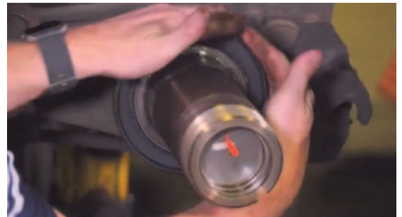
Apply lubricant being used onto OD of seal
