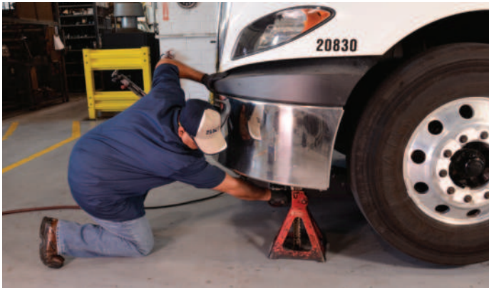
Use a proper supporting device to support the vehicle. Carefully release air spring brakes.
