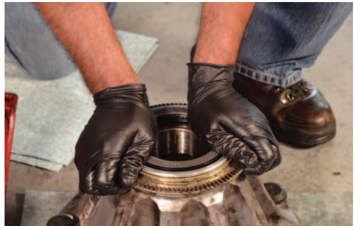
Press the seal into the bore evenly by hand
