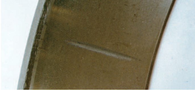
Brinelling, the result of severe impact to the bearing, causing one or more of the roller bodies to deform the surface of the race.
