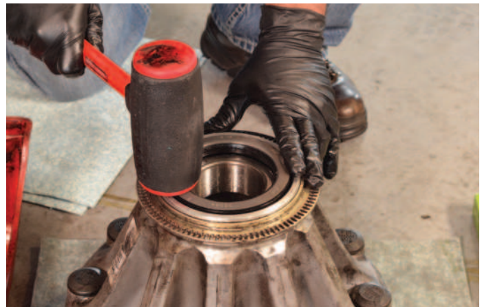
A rubber mallet may be used to tap into place
