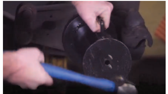
Drive seal onto spindle
