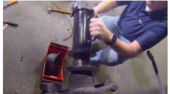
Use SKF tool 491 on spindle
