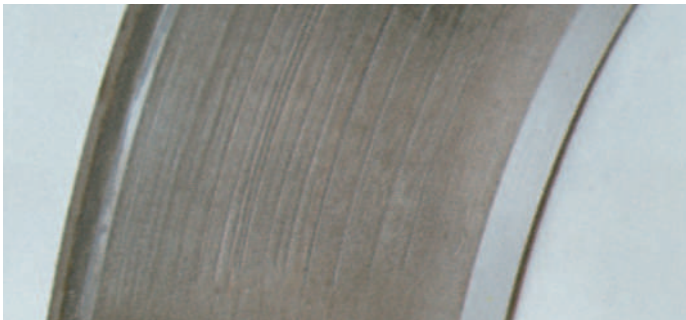
Circular wear in the race, the result of hard particle contamination in the lube.
