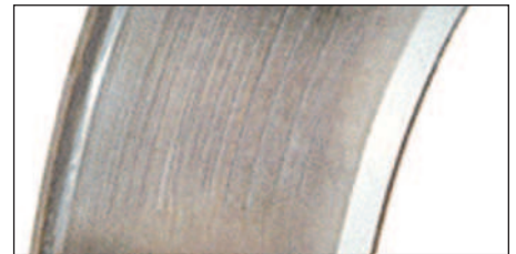
Heavy grooving by large hard particles in the lubricant.
