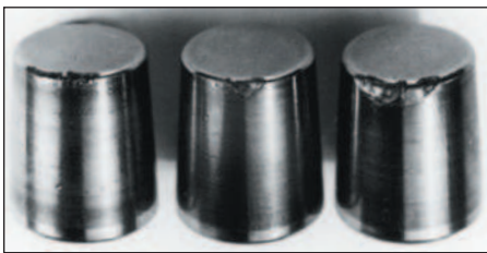
Roller end fracture due to heavy stress peaks caused by slackness of too loose bearing adjustment.
