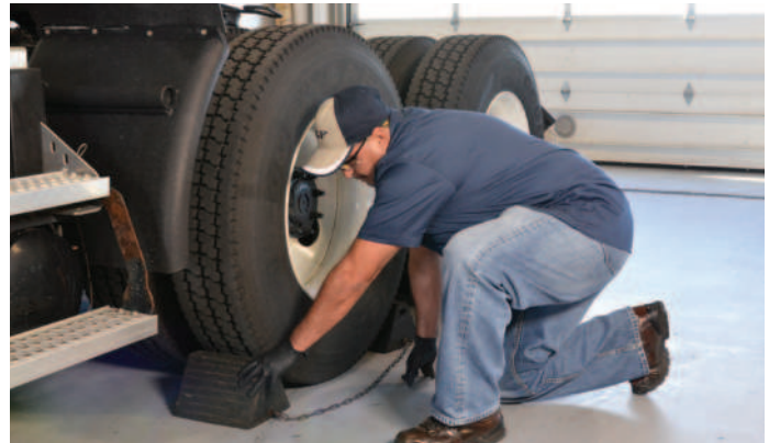
When inspecting wheel ends, be sure to block wheels and lift axle.
