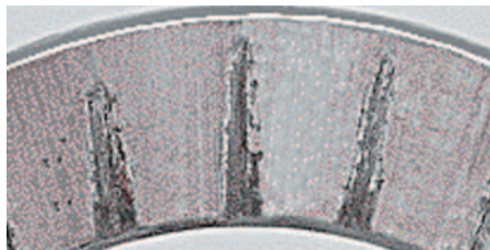
Typical surface appearance with repeated effects of vibration (called "false brinelling").
