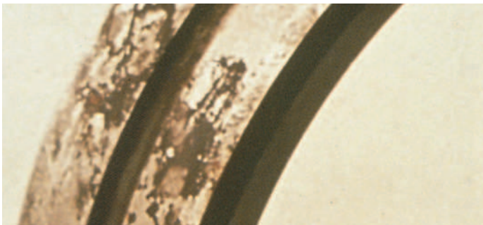
Fretting corrosion of the outer surface is often the result of a worn hub or spindle.
