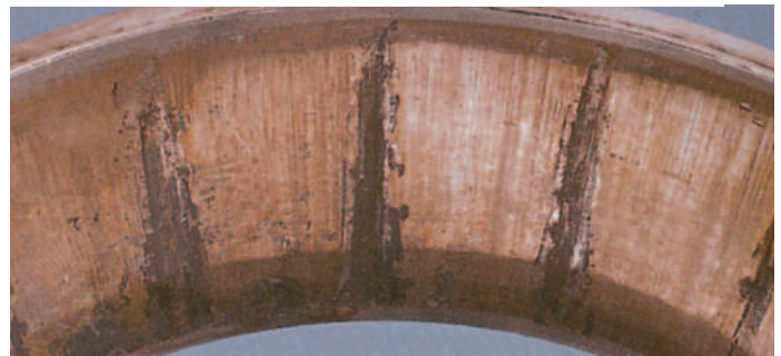
Vertical etching on the race, the result of moisture contamination within the lube.
