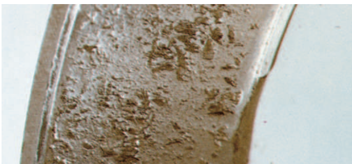
Spalling, the wearing away of metal from the bearing surface, the result of contamination, brinelling, improper installation, improper lubrication, or the normal end of bearing life.
