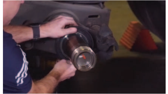
Place seal on spindle shoulder 'Oil Bearing Side' out
