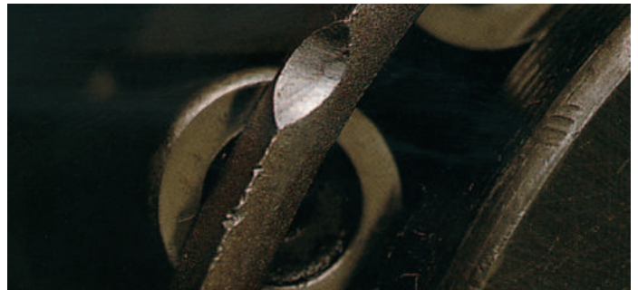
Cage damage, the result of abuse prior to or during installation.
